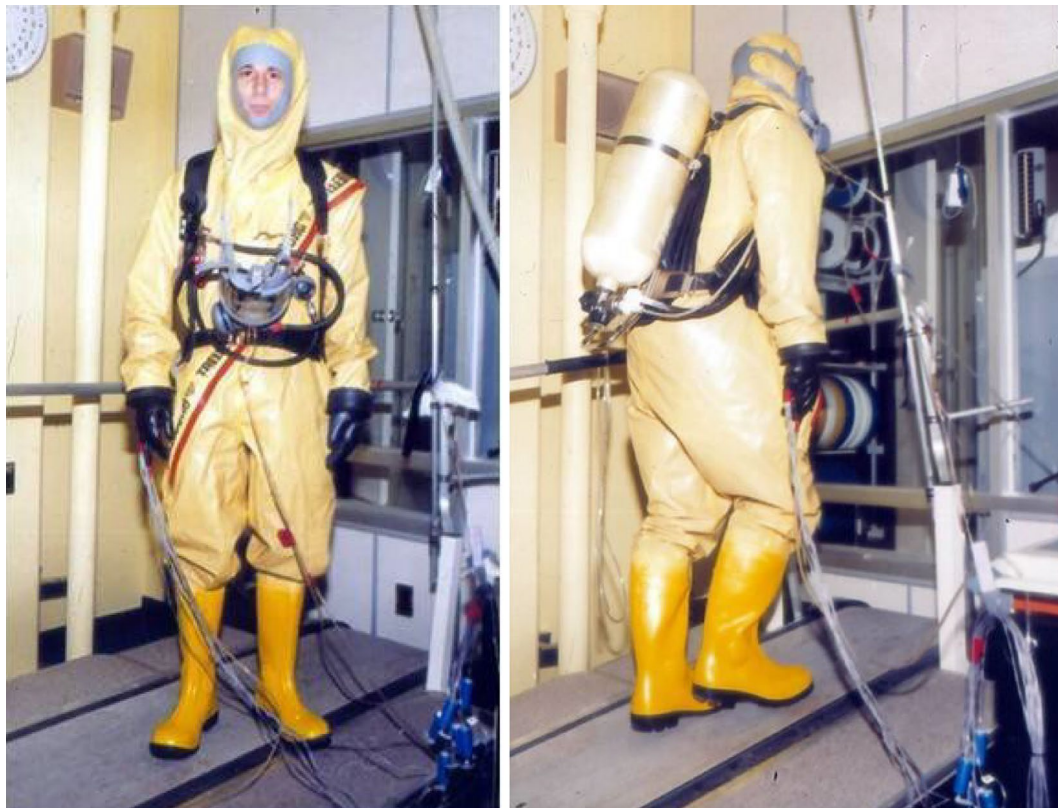
Fig. 3 Convertino performing operational tests on an impermeable ensemble during rest ( left panel ) and physical exercise ( right panel ) conducted in the summer of 1988 in the Human Physiology Laboratory at NASA's Kennedy Space Center
