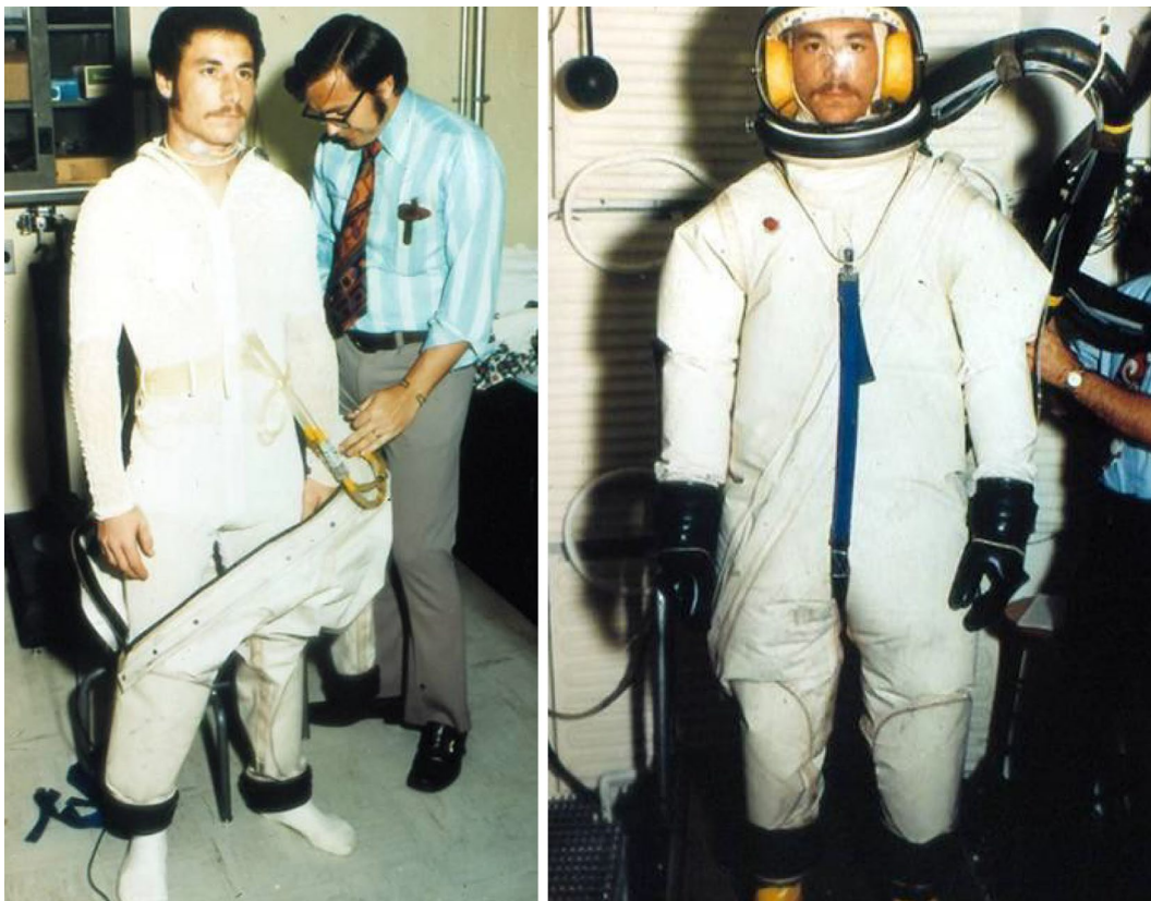
Fig. 2 Human volunteer Convertino donning an early prototype for testing of a liquid cooling garment (LCG) developed for use by astronauts for thermoregulation during extravehicular activities in the summer of 1978 at NASA's Ames Research Center. The late Dr. Alan Chambers, former Chief of the Man-Vehicle Systems Research Division and Director of Space Research, is instrumenting Convertino
