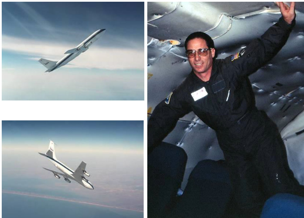
Fig. 4 25 s of 'weightlessness' produced by ascent followed by rapid descent of NASA's KC-135 aircraft ( left panels ). Convertino floating in microgravity ( free fall ) performed during January 1993 ( right panel )
