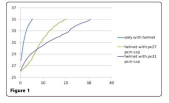
which are the products of Rubitherm company, were used. A thermocouple was used to measure temperature (°C) as a function of time (in minutes) and is presented in Figure 1.
