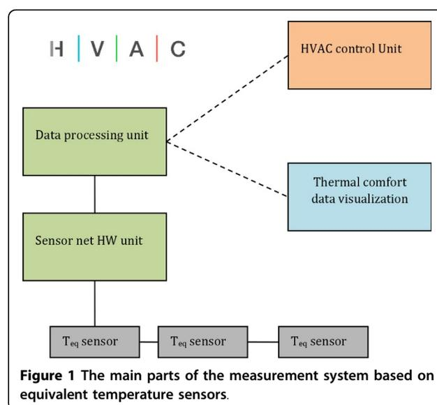
**Figure 1** The main parts of the measurement system based on equivalent temperature sensors.
