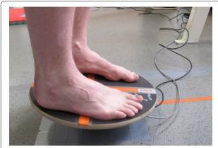
Fig. 1 Instrumented balance board used for balance tasks (L7–10).
